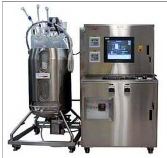
Vaccines are typically made in high volumes in heavy-duty 5,300-gallon stainless steel tanks that can take weeks to sterilize at high heat. XCellerex, launched in 2002, aims to slash manufacturing costs using so-called FlexFactories, a series of tanks one-tenth the size with disposable inserts that can be cleaned and reused more efficiently. (Forbes.com/XCellerex)
