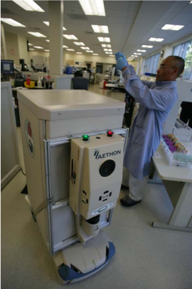
Figure 7 Typical TUG robots used for logistic support for laboratories, pharmacies and even blood banks
