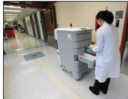
Pharmacist Trinh Nguyen takes a delivery from a TUG at Washington Hospital Center.
